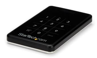
The S2510BU33PW USB 3.0 encrypted hard drive enclosure lets you to turn your 2.5-inch SATA hard drive (HDD) or solid state drive (SSD) into an AES-encrypted external drive.
