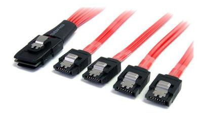
The SAS8087S4100 SFF-8087 to 4x SATA SAS cable features one 36-pin plug (SFF-8087), which fans out to four SATA 7-pin receptacles, providing a reliable solution for connecting a SATA HDD to a SAS controller or backplane.
