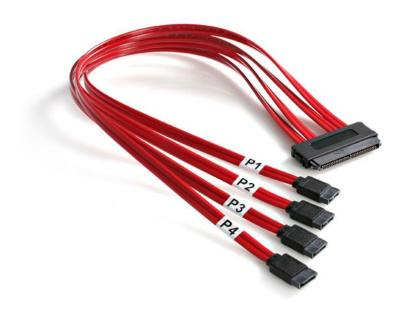
The SAS84S450 SFF-8484 to 4x SATA SAS cable features one 32-pin receptacle (SFF-8484) which fans out to four SATA 7-pin receptacles, providing a reliable solution for connecting up to four SATA HDDs to a SAS controller or backplane.
