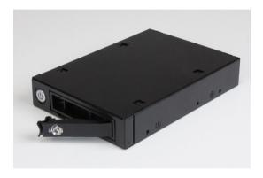
**Note:** If the drive is locked, insert either of the included bay keys into the 2.5in drive bay key hole, and turn the key clockwise into the unlock position before attempting to remove the tray.
