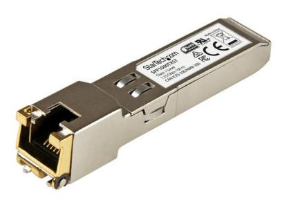
The SFP1000TXST is an MSA compliant copper SFP transceiver that's designed, programmed and tested to work with 1000BASE-TX compatible MSA switches and routers. The SFP transceiver module supports a maximum distance of up to 100 m (328 ft) and delivers dependable 1 GbE connectivity over copper cabling.
