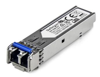
The SFP100BLXST is an MSA compliant fiber SFP transceiver that's designed, programmed and tested to work with 100BASE-LX compatible MSA switches and routers. The SFP transceiver module supports a maximum distance of up to 10 km (6.2 mi) and delivers dependable 100 Mb Ethernet connectivity over fiber cabling.
