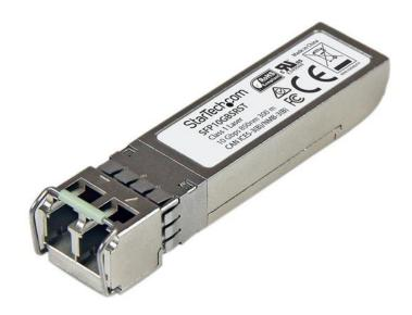
The SFP10GBSRST is an MSA compliant fiber SFP transceiver that's designed, programmed and tested to work with 10GBASE-SR compatible MSA switches and routers. The SFP+ transceiver module supports a maximum distance of up to 300 m (984 ft) and delivers dependable 10 GbE connectivity over fiber cabling.
