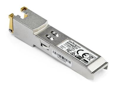
The SFP10GBTCST is a Cisco compatible copper transceiver module that has been designed, programmed and tested to work with Cisco® brand switches and routers. It delivers dependable 10 GbE connectivity over copper cable, for 10GBASE-T compliant networks, with a maximum distance of up to 30 m (98.4 ft).
