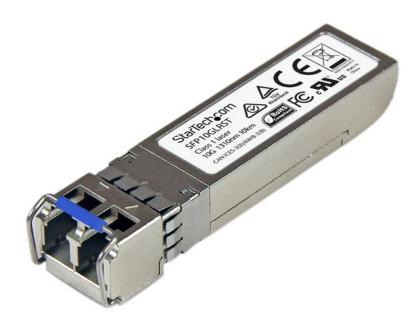
The SFP10GLRST is a Cisco SFP-10G-LR compatible fiber transceiver module that has been designed, programmed and tested to work with  $Cisco^{TM}$  brand switches and routers. It delivers dependable 10 GbE connectivity over fiber cable, for 10GBASE-LR compliant networks, with a maximum distance of up to 10 km (6.2 mi).
