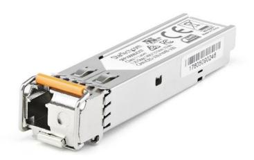
The SFP1GBX40DES is a Dell EMC SFP-1G-BX40-D compatible downstream fiber SFP transceiver which pairs with StarTech.com's SFP1GBX40UES. They are designed, programmed and tested to work with 1000Base-BX40 compatible Dell EMC switches and routers. The SFP transceiver module supports a maximum distance of up to 40 km (24.8 mi) and delivers dependable 1 GbE connectivity over fiber cabling.
