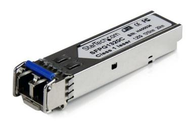
The SFPG1320C is a Cisco GLC-LH-SMD compatible fiber transceiver module that has been designed, programmed and tested to work with Cisco® brand switches and routers. It delivers dependable 1 GbE connectivity over fiber cable, for 1000BASE-LH compliant networks, with a maximum distance of up to 20 km (12.4 mi).
