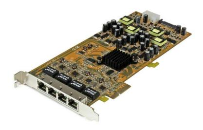
The ST4000PEXPSE 4-Port PoE NIC lets you add four Gigabit Power over Ethernet ports through a single PCI Express slot. Each port can provide up to 25.5W of power, combining network data and power over a single Ethernet cable for reduced cable clutter and added convenience for remote PoE devices.
