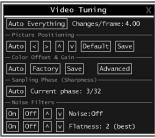
Use the **Auto Everything** button to automatically fine-tune all three adjustments. If the test pattern for Color Offset calibration is not present on the screen, then the Color Offset adjustment is skipped.
