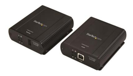
The USB2002EXT2 2-Port USB Extender lets you extend USB 2.0 devices over Cat 5 or better Ethernet cable at distances of up to 330ft (100m). A local transmitter power adapter provides up to 500 mA of power per port with no power adapter required at the remote end, letting you access and power almost any USB 2.0 device in locations where a power outlet may be unavailable.
