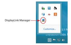
2. Click the DisplayLink icon to open the configurable options menu. A description for each configurable option is listed below.
