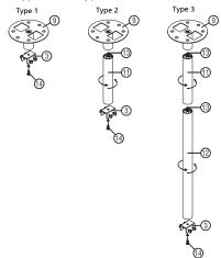
3 Type 1: For the standard size use three bracket screws to mount the projector to the ceiling mount bracket.
