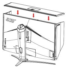
5. Shading hood installation complete.
