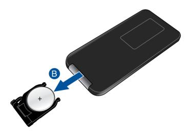
C. Remove the old battery then insert the new CR2025 lithium coin battery into the battery holder with the positive side (+) facing up.
