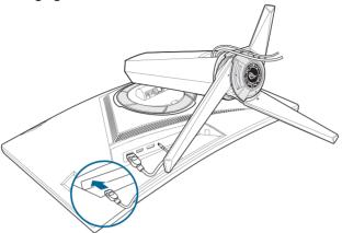
• Using the input/output port cover : the cover can be attached or detached.
