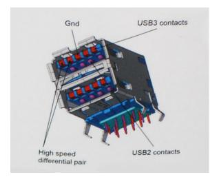
With today's ever increasing demands placed on data transfers with high-definition video content, terabyte storage devices, high megapixel count digital cameras etc., USB 2.0 may not be fast enough. Furthermore, no USB 2.0 connection could ever come close to the 480Mbps
