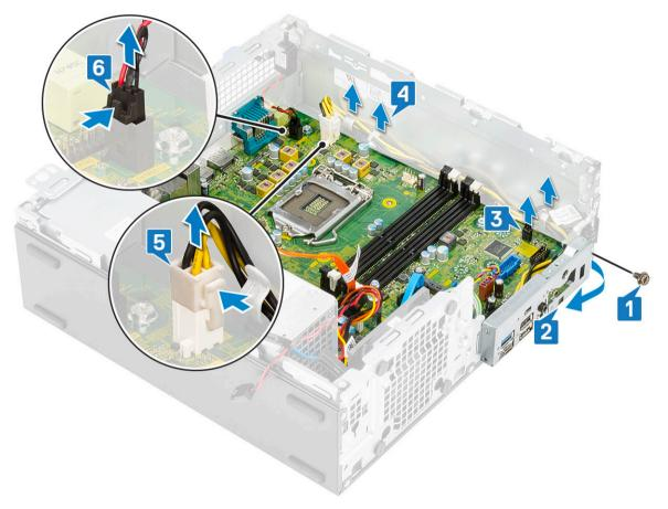
4 Disconnect the intrusion switch cable [1], PSU power cable [2], data cable [3], system fan cable [4], SATA cable [5], SATA power cable [6]
