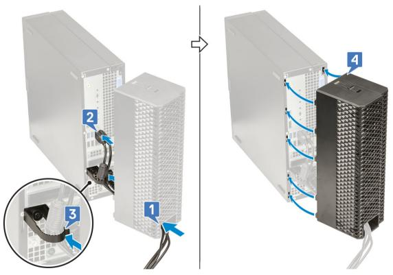
6 Gently press down on the cable cover until it clicks into place (1). Slide the latch towards the chassis (2) to lock the cable cover in place.
