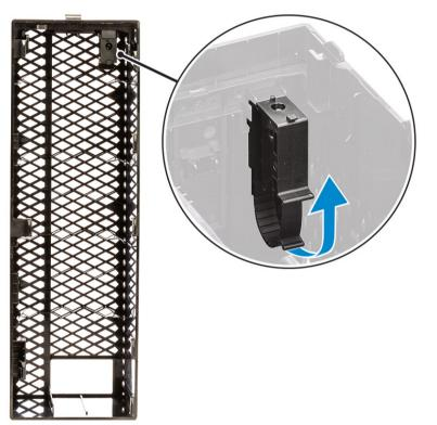
3 Lift the tab [1], to release and pull the cable tie from the slot on the cable release latch [2].
