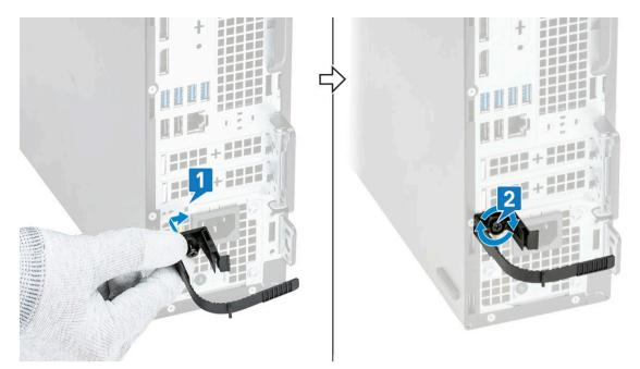
5 Route the cables through the slot of the cable cover [1], and connect them to their respective ports on the system (2). Secure the cable with the cable tie and lock the tab in place [3]. Align the plastic hooks of the cable cover to the slots on the system [4].
