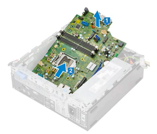
3 Replace the 5 screws that secure the system board to the system [1], the single (M3x5) screw [2], and the single (#6-32) screw [3].
