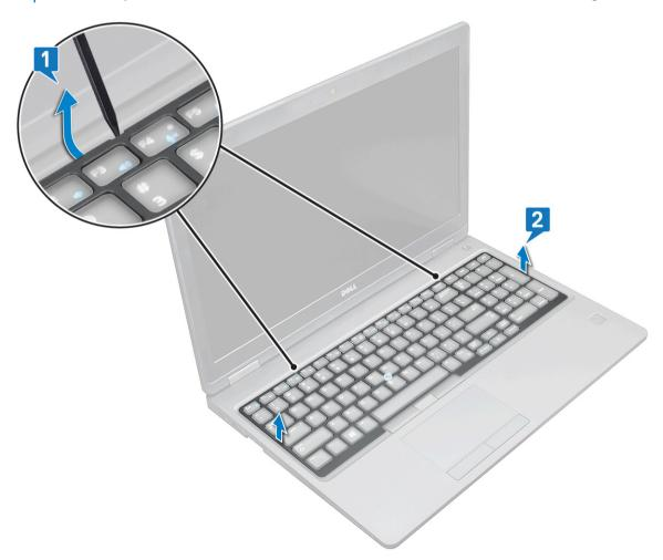
ONOTE: Use a plastic scribe to pry the keyboard lattice from the pry points and move around the lattice for removal.
