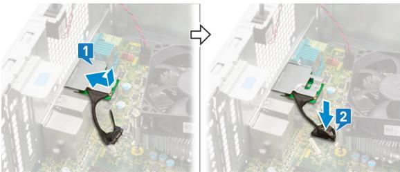
2 Replace the two (M3X3) screws to secure the optional VGA module to the system.
