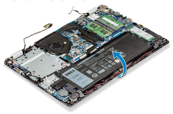
Remove the 5 M2.5x5 screws that secure the hinge brackets to palm rest [1] and lift the display assembly away from the computer [2].
