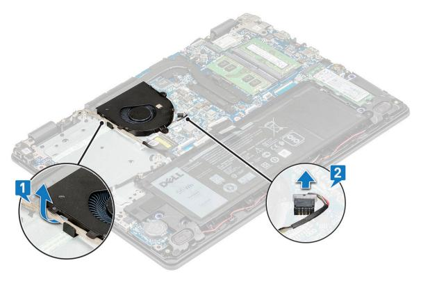
b Remove the 2 M2.5x5 screws that secure the fan to the computer [1] and lift the fan off the computer [2].
