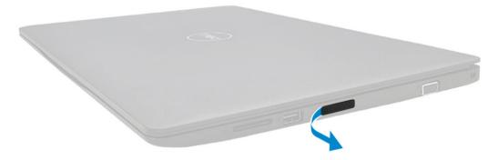
Insert the tip of a paperclip into the hole of the SIM tray slot and then pull out and remove the SIM tray.
