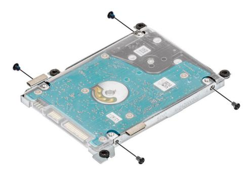
6 Lift the HDD bracket to remove it from the HDD.
