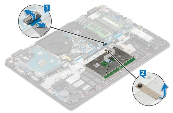
8 Remove the four M2x2 screws that secure the touchpad on the computer [1] and lift the touchpad from the system [2].
