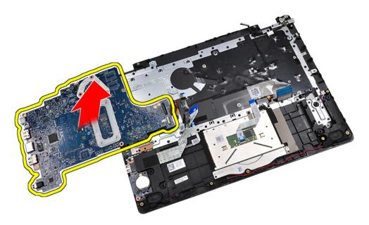
· For other configurations, flip the system board to disconnect the VGA board cable..
