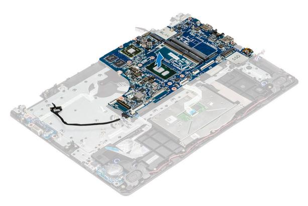
Remove the screw securing the USB Type-C bracket to the system board [1] and lift the USB Type-C bracket from the system board [2].
