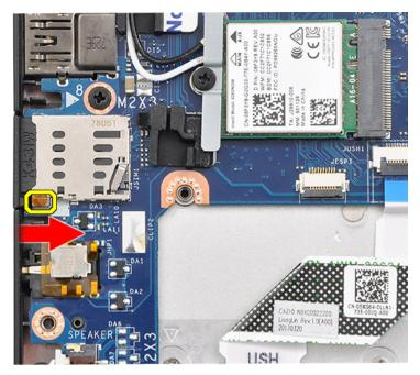
2 Slide the dummy SIM card tray out of the system.
