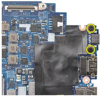
8 Flip the system board, peel off the tapes securing the bracket and remove the USB Type-C port from the system board.
