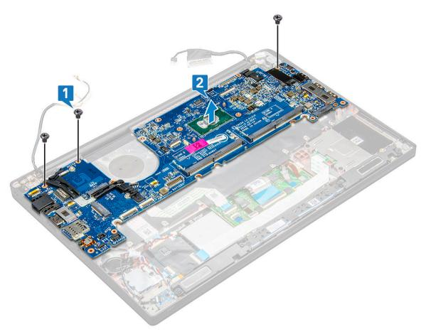
7 Remove the two (M2.0x5.0) screws that secure the USB Type-C bracket.
