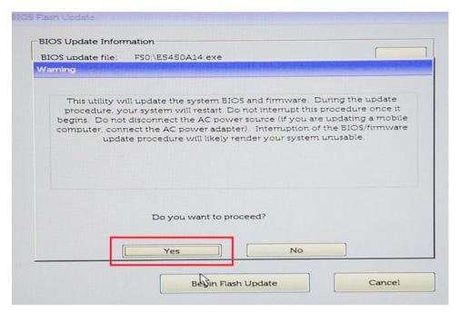
8 At this point the BIOS flash will execute, the system will reboot and then the BIOS flash will start and a progress bar will show the progress of the flash. Depending on the changes included in the update, the progress bar may go from zero to 100 multiple times and the flash process could take as long as 10 minutes. Generally this process takes two to three minutes.
