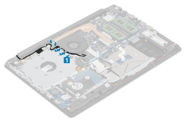
4 Connect the ODD cable, display cable and fan cable to the system board [1, 2, 3].
