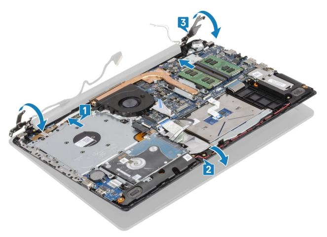
4 Replace the five (M2.5x5) screws that secure the left and right hinges to the system board, and palmrest and keyboard assembly [1].
