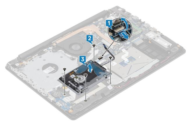
4 Disconnect the interposer from the hard drive assembly.
