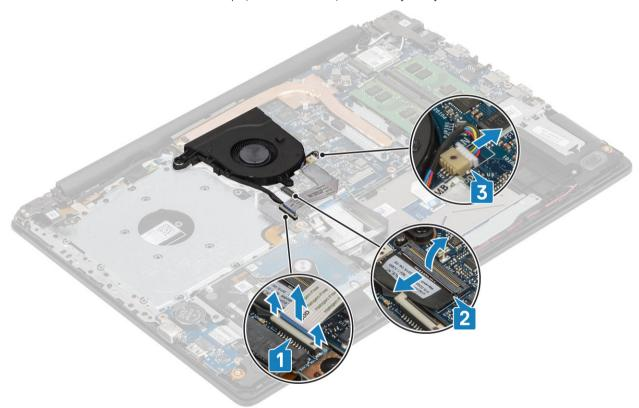
2 Unroute the display cable from the routing guides on the fan [1].
