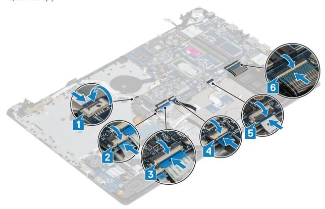
8 Connect the power adapter port cable, optical drive cable and speaker cable to the system board [1, 2, 3].
