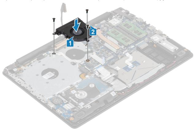
3 Route the display cable through the routing guides on the fan [1].
