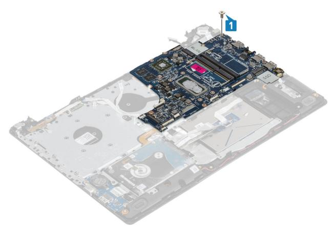
6 Place the optical drive connector and replace the single (M2x2) screw that secures it to the system board [1, 2].
