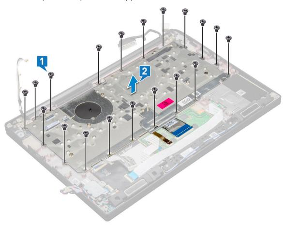
Remove the screws (5) that secures the keypad to the keyboard chassis and lift the keyboard [1,2].
