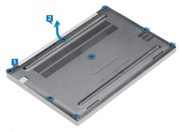
CAUTION: Exercise caution when loosening the screws. Angle the screwdriver to match the head of the screw (front corners on the laptop base cover) to avoid a possible stripped screw head.
