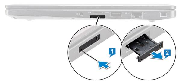
NOTE: For Latitude 7390, the SD memory card must be removed before replacing any system components. Failure to remove the SD memory card before the disassembly of other components may result in damage to the system
