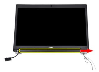
4 Remove the display hinge cap.
