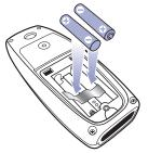
Replace the battery cover: hook the two plastic clips into place first, then lower and screw the cover into place. Finally, screw the belt clip on. You can use a coin, e.g. 10p piece if you don't have a screwdriver.
