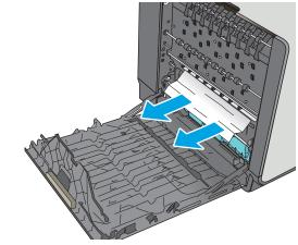
3. Remove the ink-collection unit by pulling it out with both hands. Set the unit aside, upright, on a piece of paper to prevent spills.
