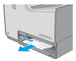
Remove any jammed or damaged sheets of paper. Verify that the tray is not overfilled and that the paper guides are adjusted correctly.
