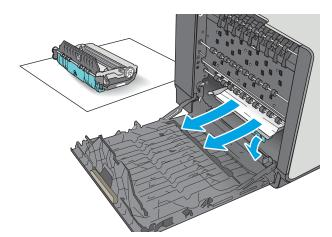
5. Lift the green tab to return the platen to the operating position.
