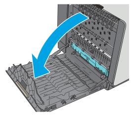
Gently pull out any jammed paper from the rollers and delivery area. If the paper tears, make sure to remove all remnants.
