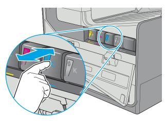
Grasp the edge of the old cartridge and then pull the cartridge straight out to remove it.
