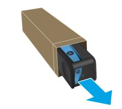
5. Do not touch the gold-colored metal contacts of the cartridge. Fingerprints on the contacts can cause print-quality problems.
