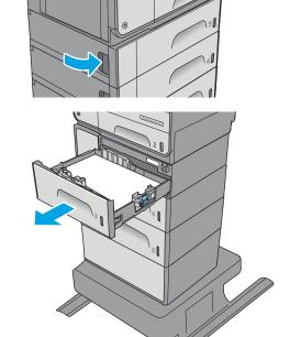
Remove any jammed or damaged sheets of paper. Verify that the tray is not overfilled and that the paper guides are adjusted correctly.
