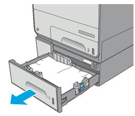
Remove any jammed or damaged sheets of paper. Verify that the tray is not overfilled and that the paper guides are adjusted correctly.
