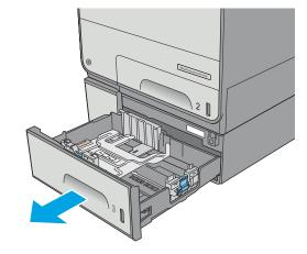
Before loading paper, adjust the paper-width guides by squeezing the adjustment latches and sliding the guides to the size of the paper being used. The edge of the tray guide should line up exactly with the marking on the tray.
