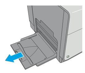
Spread the paper guides to the correct size, and then load paper in the tray. For information about how to orient the paper, see <u>Tray 1 paper</u> <u>orientation on page 19</u>.
