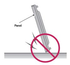
2 If the product is tilted onto the edge of the panel, the panel may be damaged.
