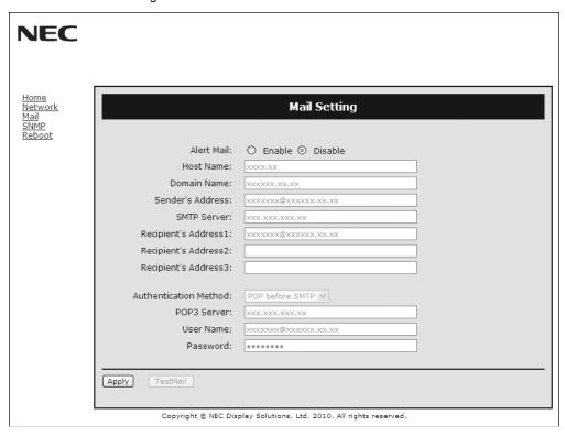
This option notifies your computer of an error message via e-mail when using wired LAN. An error message notification will be sent when an error occurs in the monitor.
