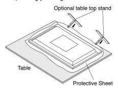
NOTE: Install the stand in the direction of the arrow which is imprinted on the surface of the stand. Use the ST-322 for V323-2.
