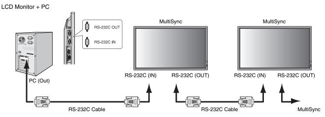
**NOTE:** If your PC is equipped only with a 25-pin serial port connector, a 25-pin serial port adapter is required. Contact your dealer for details.
