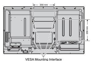
Mounting accessories can be attached with the monitor in the face down position. To avoid damaging the screen face, place the protective sheet on the table underneath the LCD. The protective sheet was wrapped around the LCD in the original packaging. Make sure there is nothing on the table that can damage the monitor.
