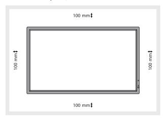
Allow adequate ventilation or provide air conditioning around the monitor, so that heat can properly dissipate away from the unit and mounting apparatus; especially when you use monitors in multiple screen.
