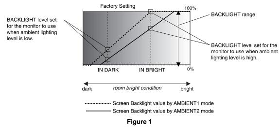
IN DARK: BACKLIGHT level set for the monitor to use when ambient lighting level is low. IN BRIGHT: BACKLIGHT level set for the monitor to use when ambient lighting level is high.
