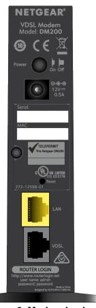
Figure 3. Modem back panel
