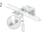
Loosen the screw so that the locking plate can slide. Then tighten to secure to the T-bar.
