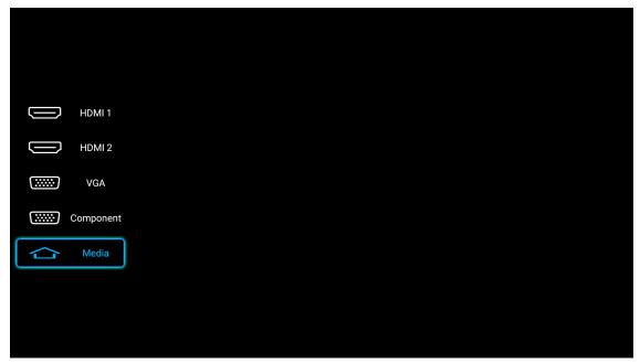
Select the desired input source and press **Enter** on the remote control or  $\leftarrow$  on the projector keypad to confirm the selection.
