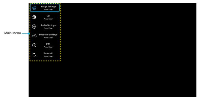
2. When OSD is displayed, use ▲▼ keys to select any item in the main menu. While making a selection on a particular page, press Enter on the remote control or - on the projector keypad to enter submenu.
