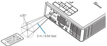
**Note:** Actual operating range may slightly differ from the diagram. Additionally, a weak battery reduces or eliminates the operating range of the remote control.
