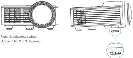
**Important Note:** To avoid damaging the projector, ensure that the adjustment wheels are fully retracted before moving the projector or placing the projector in its carrying case.
