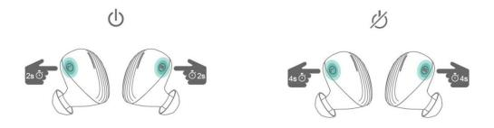
When your BE Free8 is in OFF state, press Power/Function button for about 2 seconds until the LED indicator flashes white and you hear the "Power on" on your left earpiece.
