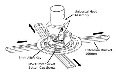
2A.2— Place projector's Flush Mount Assembly over the projector and align the centre of the Flush Mount with the projector's approximate Centre of Gravity.
