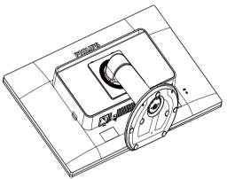
2. Remove the screws from hinge cover.
