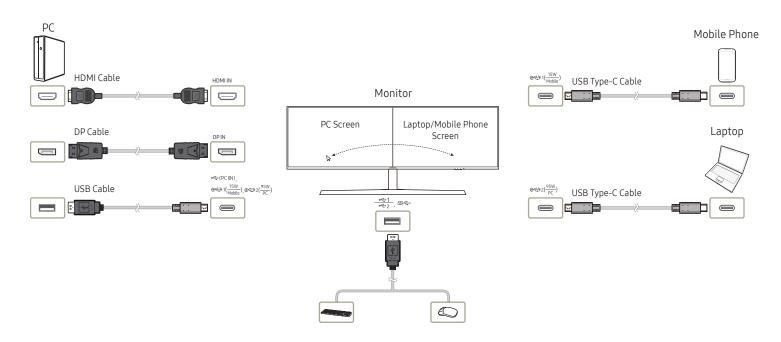
The KVM (keyboard, video, and mouse) switch enables users to use only a keyboard, a video monitor, and a mouse for controlling multiple input sources.
