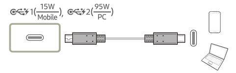
The USB Type-C port can support USB Power Delivery, Data, and DP video signal.
