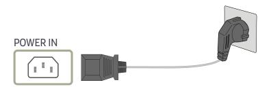
To use the product, connect the power cable to a power outlet and the **POWER IN** port on the product.
