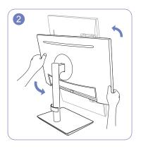
Rotate the machine to the highest vertical position.
