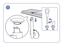
Insert the stand neck into the stand base in the direction shown in the figure. Tightly fasten the connecting screw at the bottom of the stand base.
