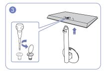
Lift the stand neck in the arrow direction to detach it Unfasten the connecting screw at the bottom of the stand base, and then remove the stand neck from the stand base by pulling it in the arrow direction, as shown in the figure.
