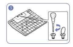
Tightly fasten the connecting screw at the bottom of the stand base.
