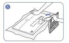
Insert the stand head into the connection hole in the direction, as shown in the figure.
