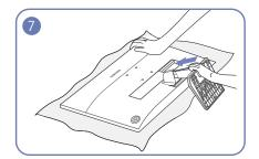
Push the assembled stand into the main body in the direction of the arrow, as shown in the figure.
