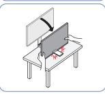
• Do not put any object under the product. There is a risk of damage to the object when lowering the product close to the floor.
