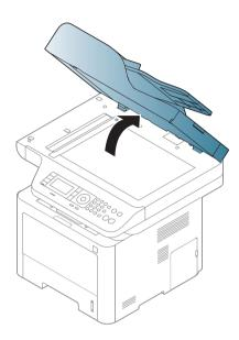
Place the original face down on the scanner glass. Align it with the registration guide at the top left corner of the glass.
