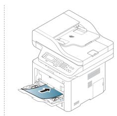
Squeeze the multi-purpose (or manual feeder) tray paper width guides and adjust them to the width of the paper. Do not force them too much, or the paper will bent resulting in a paper jam or skew.
