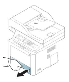
2 Squeeze and the paper width guide and paper length lever to locate them in the correct paper size slot marked at the bottom of the tray to adjust to the size (see "Tray overview" on page 47).
