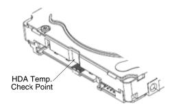
Figure 1 Location of the HDA temperature check point
