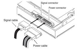
Each cable is keyed to ensure correct orientation. Desktop HDD drives support latching SATA connectors.
