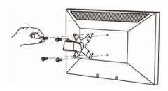
**WARNING!** Do not over-tighten the screws and stop immediately if you encounter resistance to avoid damage to your display. Ensure that all spacers and screws being used are the same length and thread type.
