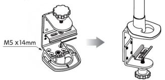
4. Place the EVA Cushion (4) beneath the Support Post (1) and then place the Desk Clamp opening around the edge of your desktop in your desired location. Tighten by hand to secure, ensuring that the clamp is making full contact with the desk surface.
