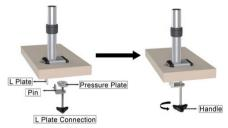
3. Loosen the collar on the support post and adjust to the desired height.
