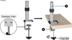
**Grommet Clamp:** Place the L Plate through the grommet hole of your desk surface, then attach the bottom portion of the Clamp **(4)** to the L Plate and tighten by hand to secure. Ensure that the Clamp is making full contact with the desk surface.
