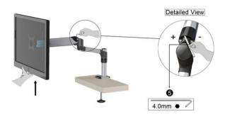
To increase / decrease the tilt resistance, adjust the set screw located on the side of the Mount Bracket joint, using the 6mm Allen Wrench (6).
