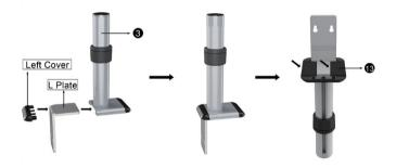
Desk Clamp: Attach the bottom portion of the Clamp (4) to the L Plate, then place
