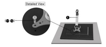
**WARNING!** Do not over-tighten the screws and stop immediately if you encounter resistance to avoid damage to your display. Ensure that all spacers and screws being used are the same length and thread type.
