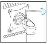
Adjusting the Swivel Tension
