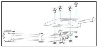
Thread the Four M5 Nuts onto the M5x12 Screws
