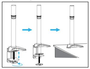
Attaching the Clamp to a Surface
