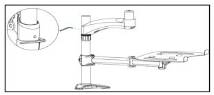
Adjusting the Swivel Tension
