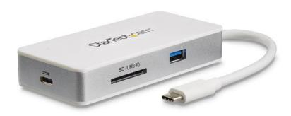
Expand the connectivity of your Thunderbolt<sup>TM</sup> 3/USB-C<sup>TM</sup> port enabled laptop. Compatible with Mac and Windows, this universal USB-C multiport adapter lets you turn your laptop into a powerful workstation, anywhere you go. The USB-C adapter provides a 4K Ultra HD HDMI® video output, an ultra high-speed SD<sup>TM</sup> 4.0 card reader (with UHS-II support), a USB 3.0 Type-A port and one Gigabit Ethernet port, through your laptop's USB-C port.
