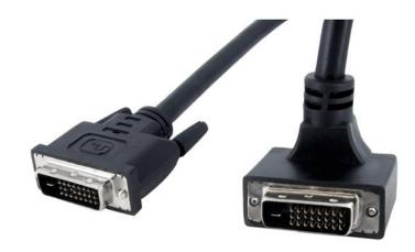
The DVIDDMMBA6 6ft Dual Link DVI-D cable features a standard DVI-D dual link connector as well as a DVI-D dual link connector that is situated on an downward angle relative to the shaft of the cable, requiring only 40mm of space at the connection point.
